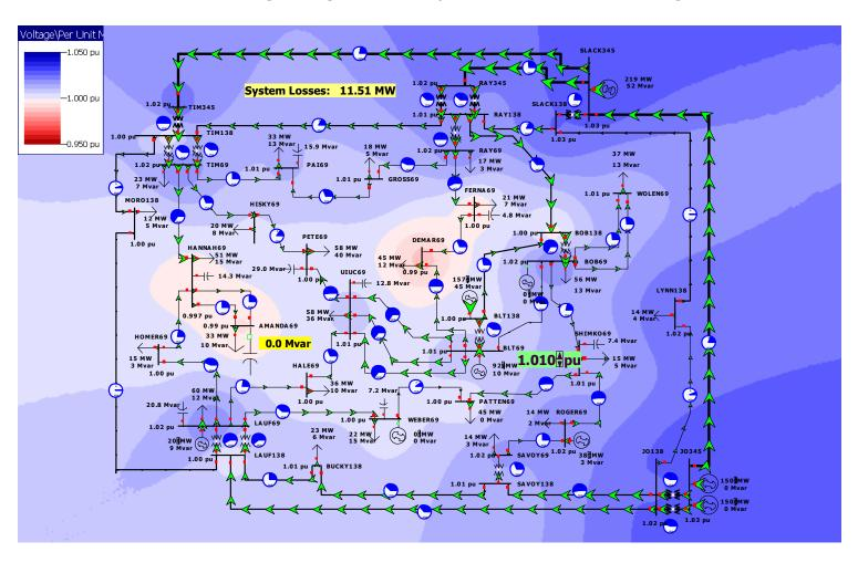
Display shows voltage contour of the power system
