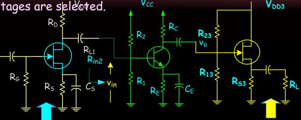
Self bias CS Amp. To provide very high Rin but small signal V<sub>o</sub> since it is a preamplifier stage Take  $A_V = -12$
