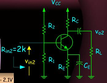
Designed  $R_1 = 19.25 k\Omega$ ,  $R_2 = 72.57 k\Omega$   $I_C = 2.94 mA$
