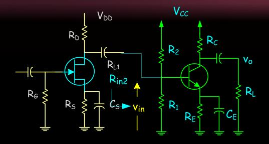
Self Bias CS Amp.  $R_G = 20M\Omega$ ,  $A_v = -12$  and  $R_D$ =  $R_{L1}$  =  $R_{in2}$  =  $2k\Omega$ . Assume  $R_C$  =  $R_L$  =  $2k\Omega$ ,  $R_E$  =  $0.4k\Omega$  $V_{D} = V_{DD} / 2 = 10V$
