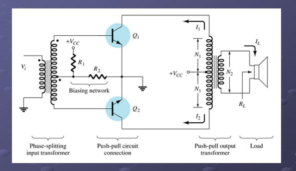
Each transistor produces one-half of an AC cycle. The transformer combines the two outputs to form a full AC cycle.
