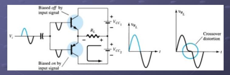
Cross over distortion can be eliminated the by biasing the transistors in class AB operation where the transistors are biased to be on for slightly more than half a cycle
