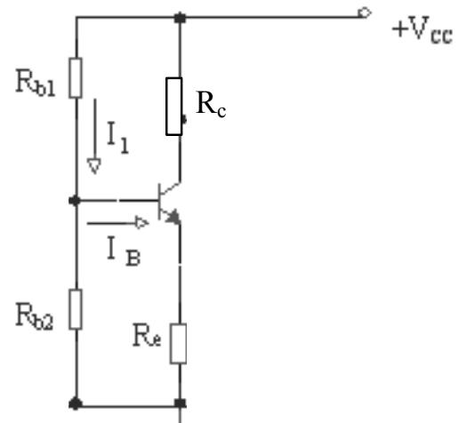
$$V_B - V_{BE} = I_E R_e \quad V_B = \frac{V_{CC}}{R_{b1} + R_{b2}} R_{b2} \quad I_C \approx I_E = \frac{V_B - V_{BE}}{R_e} \approx \frac{V_B}{R_e}$$
