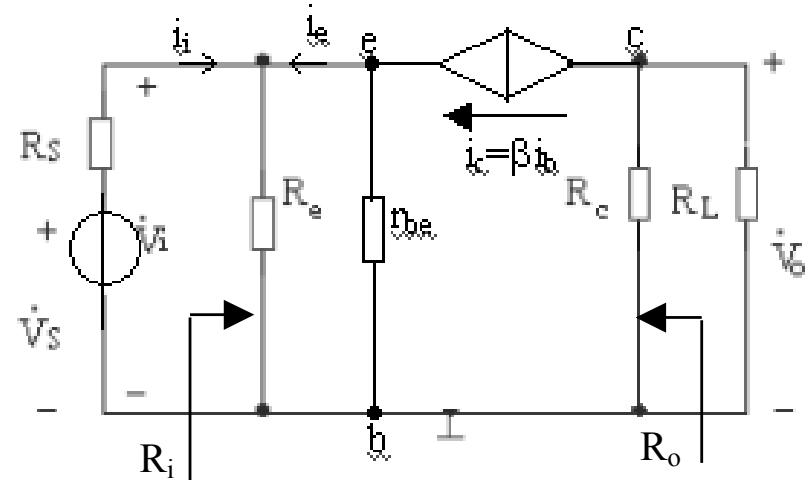
$$\rightarrow A_v = \frac{-i_c(R_c // R_L)}{-i_b r_{be}} = \frac{\beta(R_c // R_L)}{r_{be}}$$
