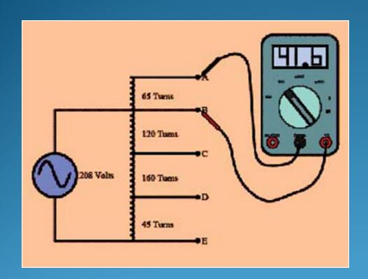
The amount of voltage across terminals A and B can be determined by multiplying the number of turns by the volts per turn of the transformer.
