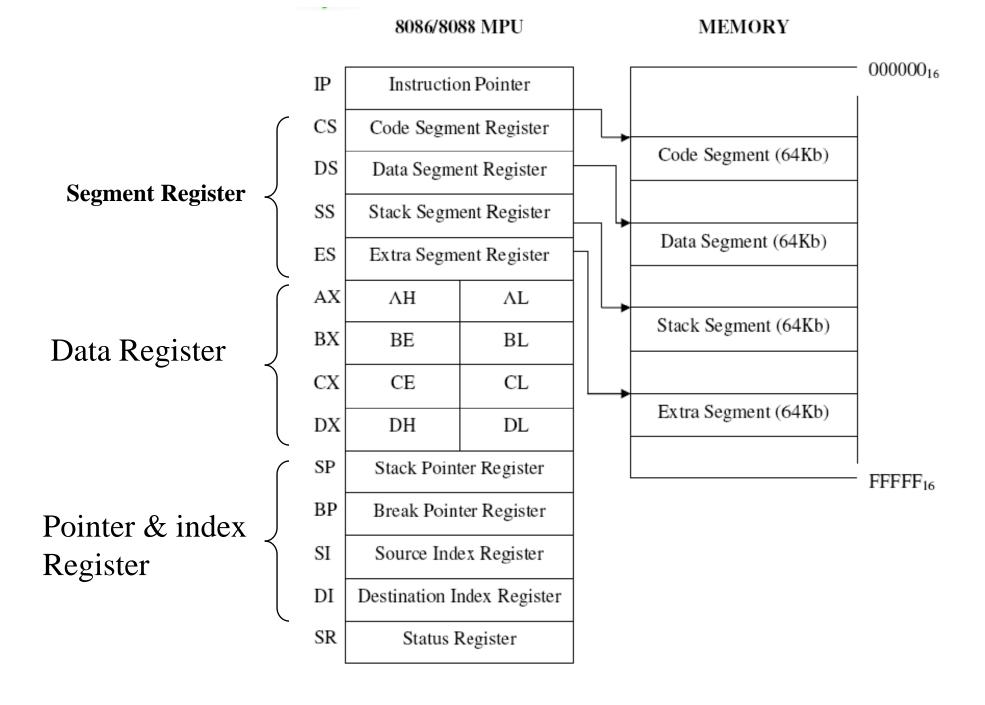
**Data segment** (DS) is a 16-bit register containing address of 64KB segment with program data. By default, the processor assumes that all data referenced by general registers (AX, BX, CX, DX) and index register (SI, DI) is located in the data segment. DS register can be changed directly using POP and LDS instructions.
