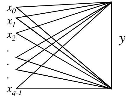
$$C = \max_{P(x_i)} (I(X;Y)) = \max_{P(x_i)} \left( \sum_{i=0}^{q-1} \int_{-\infty}^{\infty} P(X = x_i) p(Y = y | X = x_i) \log \frac{p(Y = y | X = x_i)}{p(Y = y)} dy \right)$$
