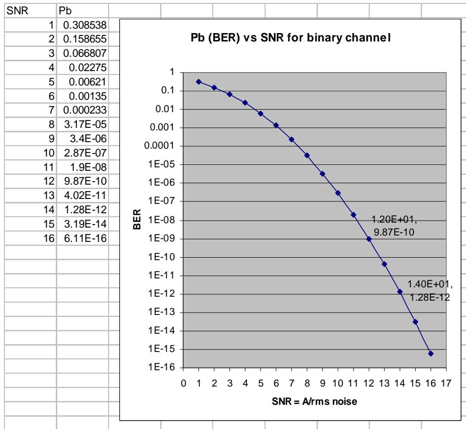
$$P_b = \frac{1}{2} \operatorname{erfc} \left( \frac{1}{2} \frac{\text{Amplitude}}{\sqrt{2} \text{ rms noise}} \right)$$
