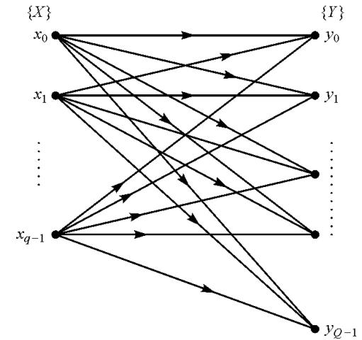
$$\begin{aligned} I(X;Y) &= \sum_{j=0}^{q-1} \sum_{i=1}^{Q-1} P(X = x_j) P(Y = y_i | X = x_j) \log \frac{P(Y = y_i | X = x_j)}{P(Y = y_j)} \\ &\equiv \sum_{j=0}^{q-1} \sum_{i=1}^{Q-1} P(x_j) P(y_i | x_j) \log \frac{P(y_i | x_j)}{P(y_j)} \end{aligned}$$
