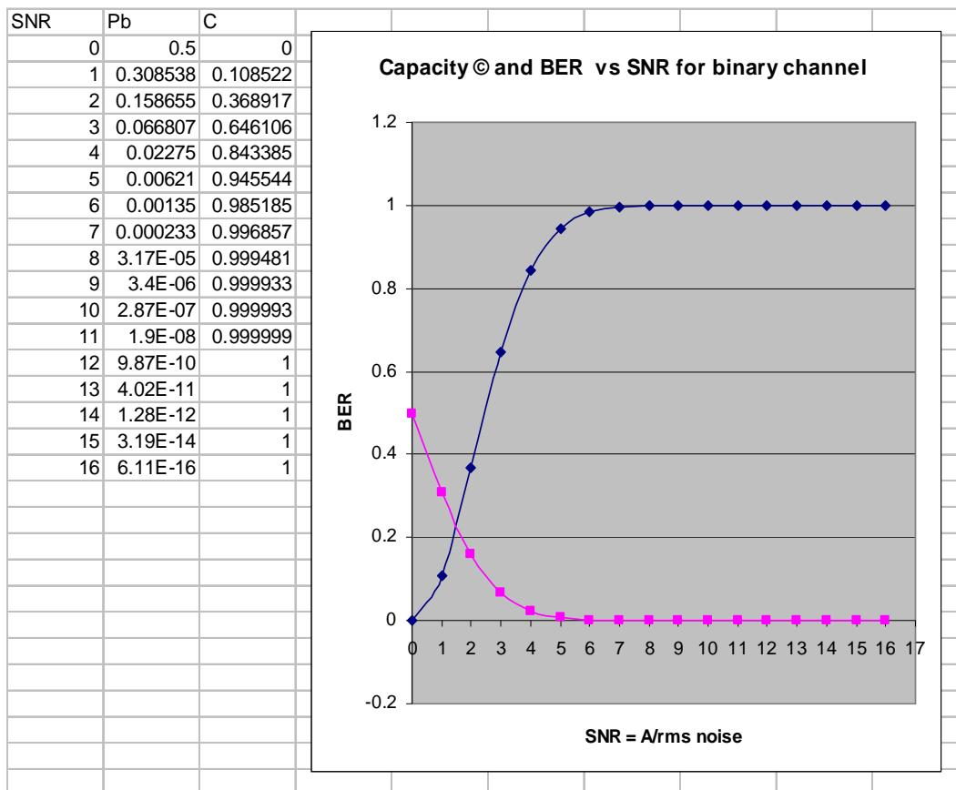
$$P_b = \frac{1}{2} \operatorname{erfc} \left( \frac{1}{2} \frac{\text{Amplitude}}{\sqrt{2} \text{ rms noise}} \right)$$
