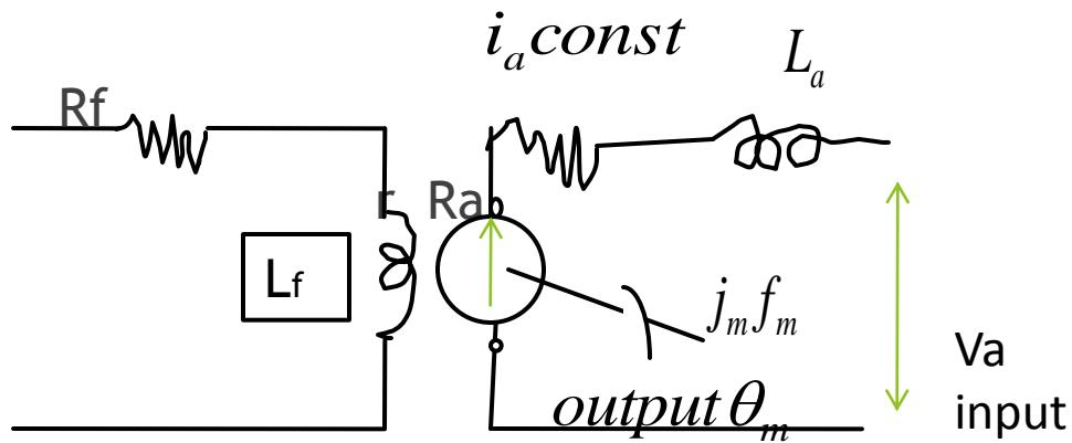
Armature controlled DC motor
