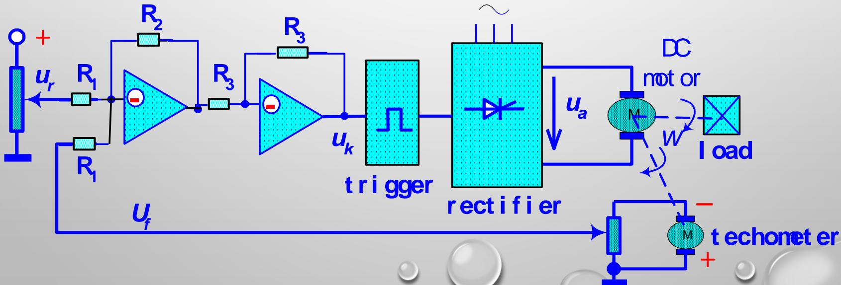
$$[T_e T_m s^2 + T_m s + (1 + k_1 k_2 \alpha \frac{1}{C_e})] \Omega(s) = k_1 k_2 \frac{1}{C_e} U_r(s) - \frac{T_e T_m s + T_m}{J} \bar{M}(s)$$
