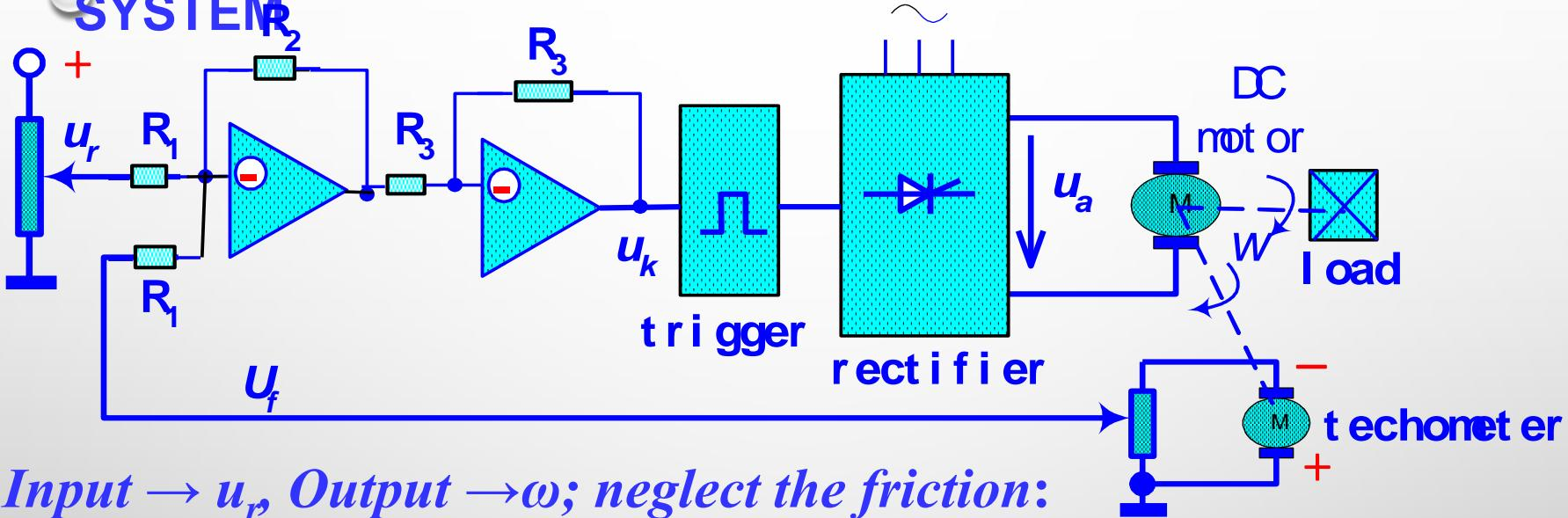
*Input  $\rightarrow u_r$ , Output  $\rightarrow \omega$ ; neglect the friction:*
