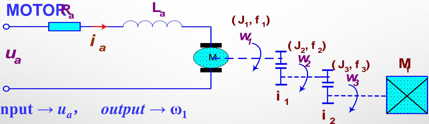
$$L_a \frac{di_a}{dt} + R_a i_a + E_a = u_a \dots \text{(1)} \quad (4) \rightarrow (2) \rightarrow (1) \text{ and } (3) \rightarrow (1) :$$
