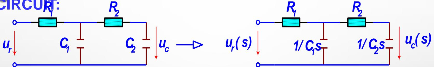
$$U_c(s) = \frac{\frac{1}{sC_1} / \left( R_2 + \frac{1}{sC_2} \right)}{R_1 + \frac{1}{sC_1} / \left( R_2 + \frac{1}{sC_2} \right)} \cdot U_r(s) \cdot \frac{\frac{1}{sC_2}}{R_2 + \frac{1}{sC_2}}$$
