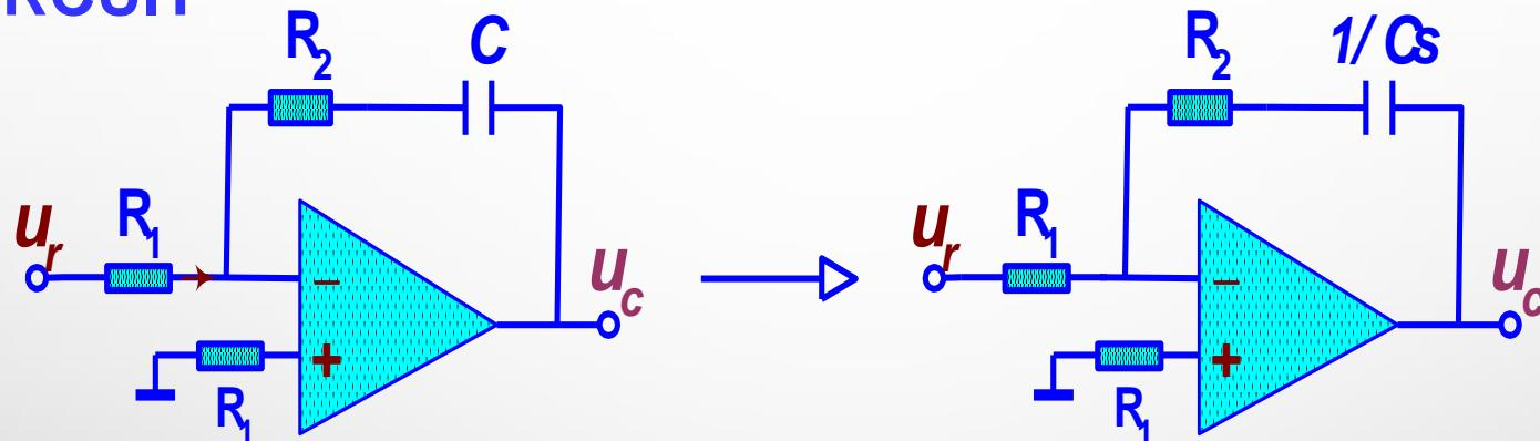
$$G(s) = \frac{U_c(s)}{U_r(s)} = -\frac{R_2 + \frac{1}{sC}}{R_1} = -\frac{R_2 Cs + 1}{R_1 Cs}$$
