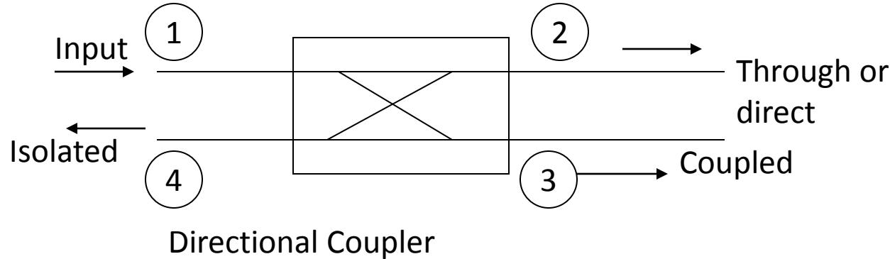
$$\text{Coupling} = C = 10 \log \frac{P_1}{P_3} = -20 \log \beta \text{ dB}$$
