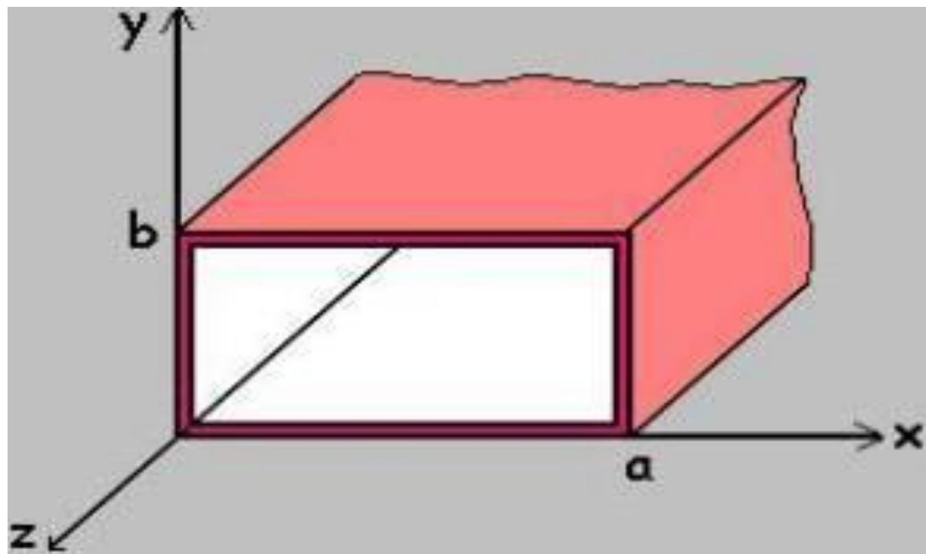
$$\frac{\partial^2 E_z}{\partial x^2} + \frac{\partial^2 E_z}{\partial y^2} + (\gamma^2 + \omega^2 \mu \epsilon) E_z = 0$$
