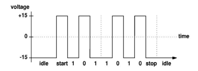
Serial communications does not have to use 7 bits of length. As a matter of fact, a whole variety of start and stop bit patterns and bit lengths can be used.
