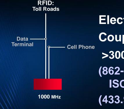
Electromagnetic Field Coupling: Lower Range UHF >300 MHz <3 (<1) GHz (862-928 MHz ANSI MH10.8.4, ISO 18185, B-11 & GTAG) (433.92 MHz ISO 18185)
