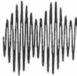
The input to the diode detector from the last IF amplifier
