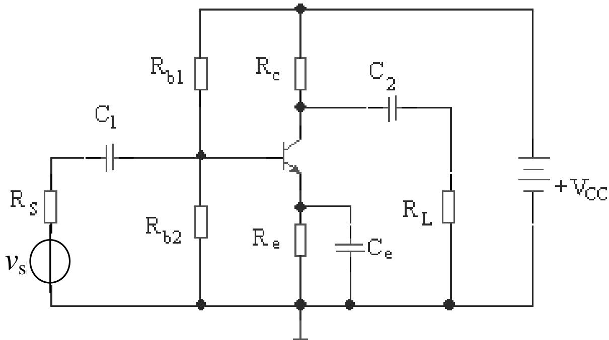
$$V_B = \frac{R_{b2}}{R_{b1} + R_{b2}} V_{CC}$$
