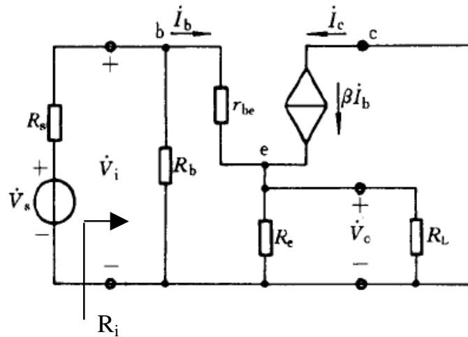
$$v_i = i_b r_{be} + i_e (R_e // R_L) = i_b [r_{be} + (1 + \beta)(R_e // R_L)]$$
