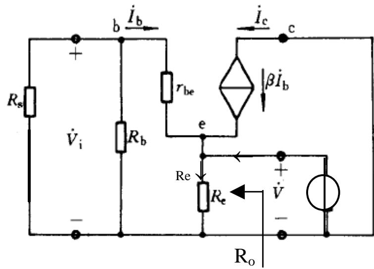
$$R_i = [r_{be} + (1 + \beta)(R_e // R_L)] // R_b$$
