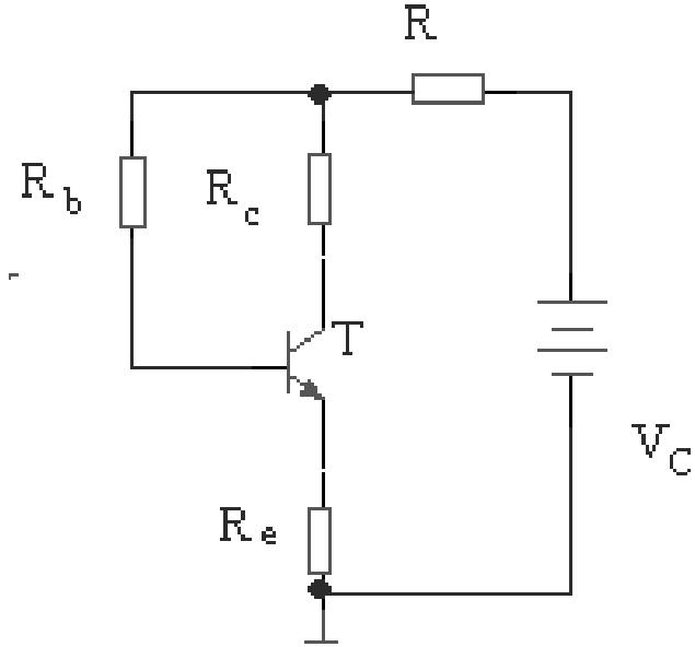
$$V_C = (I_B + I_C)R + I_B R_b + V_{BE} + I_E R_e$$
