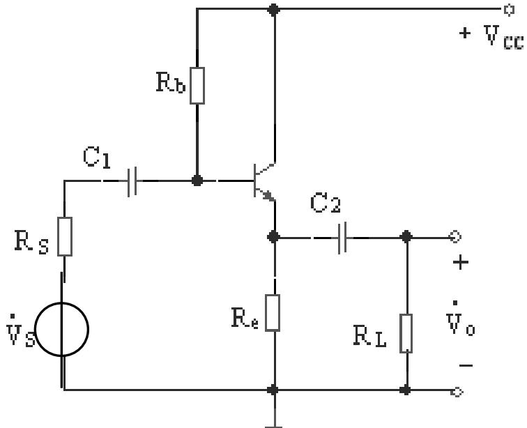
$$V_{CC} = I_B R_b + V_{BE} + I_E R_e = I_B R_b + V_{BE} + (1 + \beta) I_B R_e$$
