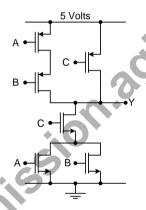
(A)  $Y = \overline{A} \overline{B} + \overline{C}$ (C)  $Y = (\overline{A} + \overline{B}) \overline{C}$
