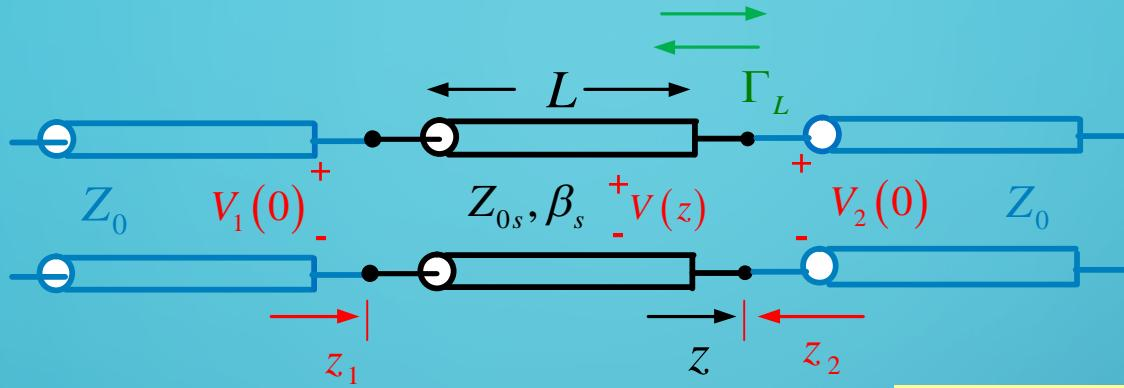
$$V_2^-(0) = \frac{V_1(0)}{e^{+j\beta_s L} (1 + \Gamma_L e^{-j2\beta_s L})} (1 + \Gamma_L)$$
