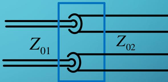
$$S_{21} = \left. \frac{b_2(0)}{a_1(0)} \right|_{a_2=0} = \left. \frac{\frac{V_2^-(0)}{\sqrt{Z_{02}}}}{\frac{V_1^+(0)}{\sqrt{Z_{01}}}} \right|_{a_2=0}$$
