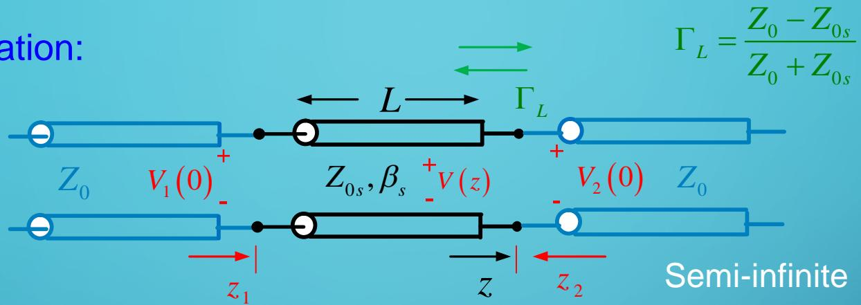
$$S_{11} = \left. \frac{b_1}{a_1} \right|_{a_2=0} = \frac{Z_{in}|_{a_2=0} - Z_0}{Z_{in}|_{a_2=0} + Z_0} = S_{22} \text{ (by symmetry)}$$
