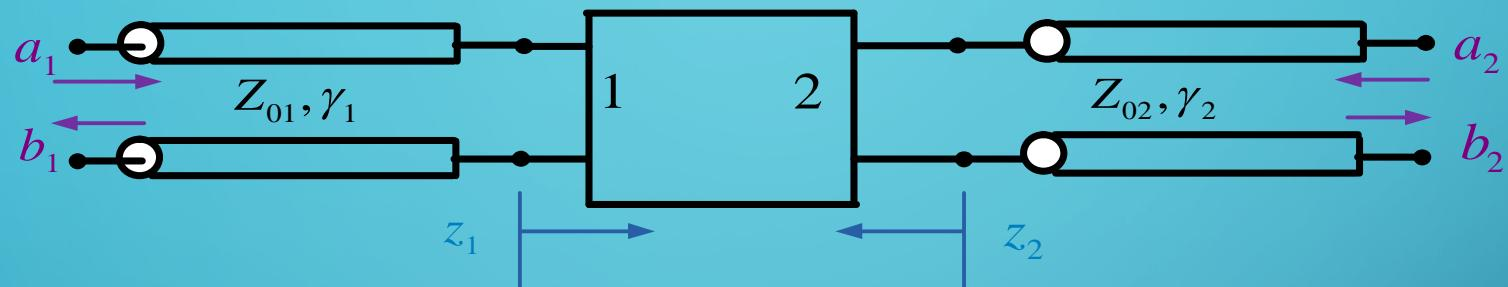
$$P_i^+(0) = \frac{1}{2} \operatorname{Re} [V_i^+(0) I_i^{+*}(0)] = \frac{1}{2} \frac{|V_i^+(0)|^2}{Z_{0i}} \quad (\text{assuming lossless lines})$$
