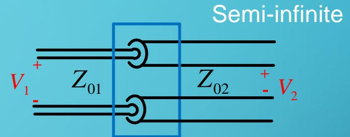
$$S_{21} = \left. \frac{\frac{V_2^-(0)}{\sqrt{Z_{02}}}}{\frac{V_1^+(0)}{\sqrt{Z_{01}}}} \right|_{a_2=0} = \left. \frac{\frac{V_1^+(0)(1 + S_{11})}{\sqrt{Z_{02}}}}{\frac{V_1^+(0)}{\sqrt{Z_{01}}}} \right|_{a_2=0}$$
