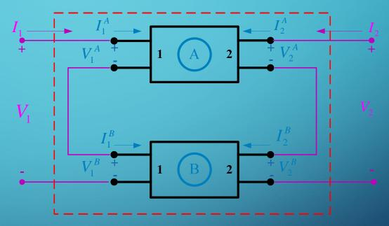
$$\begin{bmatrix} V_1 \\ V_2 \end{bmatrix} = \begin{bmatrix} Z_{11}^A + Z_{11}^B & Z_{12}^A + Z_{12}^B \\ Z_{21}^A + Z_{21}^B & Z_{22}^A + Z_{22}^B \end{bmatrix} \begin{bmatrix} I_1 \\ I_2 \end{bmatrix}$$
