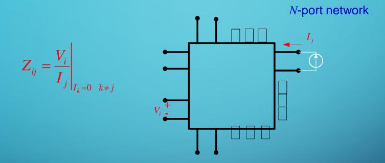
We inject a current into port j and measure the voltage (with an ideal voltmeter) at port i. All ports are open-circuited except j.
