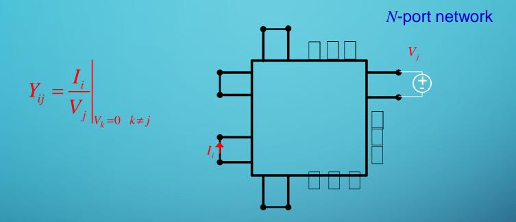
We apply a voltage across port j and measure the current (with an ideal current meter) at port i. All ports are short-circuited except j.
