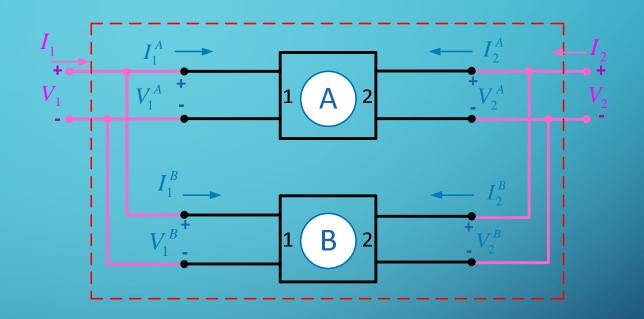
$$= \begin{bmatrix} Y_{11}^A + Y_{11}^B & Y_{12}^A + Y_{12}^B \\ Y_{21}^A + Y_{21}^B & Y_{22}^A + Y_{22}^B \end{bmatrix} \begin{bmatrix} V_1 \\ V_2 \end{bmatrix}$$
